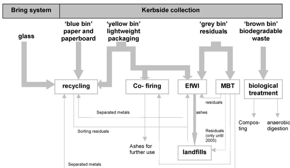
**Fig. 3.** Illustration of the present German MSW management system since the tightened waste acceptance criteria for landfill sites came into force in 2005 (Dehoust et al., 2005).
